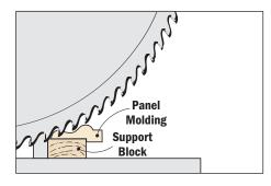
Now turn on the saw and lower the spinning blade until it cuts all the way through the molding and the support block. Repeat the process for the other end of the molding by rotating the turntable to the opposite 45° angle setting.
