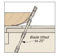
**Step 2** — Flip the workpiece around and place it flat on the table to make your second cut.
