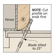
**Step 1** — Tilt the saw blade to approximately 25° and position the workpiece vertically to make the first cut. Start on edges with end grain to avoid tearout.
