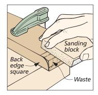
**Step 3** — Sand or plane away the remaining waste to smooth out the roundover and complete the profile.
