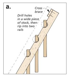
Next, partially drive a small nail or screw into each end of the shelf, somewhere near the back. Now simply hang the shelves from the half circles you created in the rails. With the rack leaning against a wall, you can finish and hang several shelves at the same time without taking up a lot of space.
