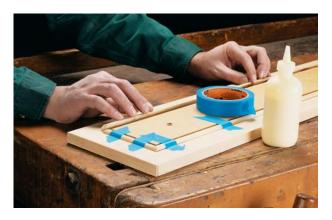
To avoid accidentally gluing the jig to the false front, I waxed the edges of the jig.
