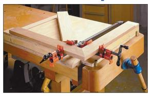
Whenever I'm assembling mitered frames, I have a difficult time holding the frame pieces in position while gluing or installing fasteners. But instead of buying an expensive corner clamp, I made my own using a couple of pipe clamps.
