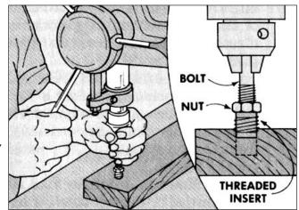
When the insert is completely embedded, lock the spindle in place and back off the nut from the top of the insert. Then unlock the spindle and unthread the bolt from the insert while slowly releasing pressure on the control arm.
