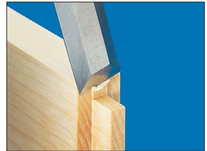
Remove stepped shoulders with a chisel.
