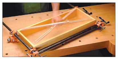
I solved this problem by making an adjustable squaring gauge, as shown in the photo above. The gauge is simply an adjustable length of wood that I can use to compare the inside diagonals of a cabinet. By sliding the pieces together or apart, I can adjust the length to fit a variety of different projects. An L-shaped hook at each end fits precisely into the corners, and a small cam device allows me to lock-in my first diagonal measurement.
