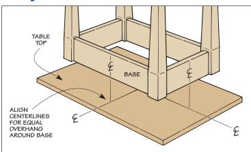
apron (or side), making a mark on the outside face of each one where it meets the top. Once the centers are marked, place the base upside down on the table top.
