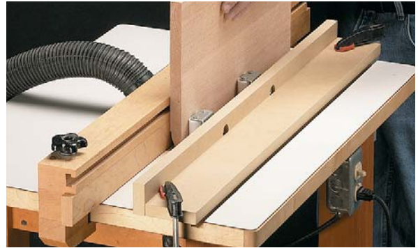
A spring adds pressure, while the roller lets the workpiece glide by.
