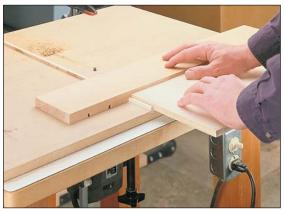
Next I inset a strip of wood into the top to serve as an index pin for spacing the dadoes, see Figure 1. I made sure that the distance between the router bit and the index pin equaled the spacing I needed for my dadoes, then I clamped the top to my router table.
