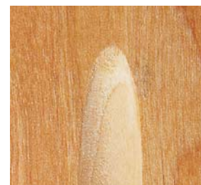
▲ The ramps lift the bit out of the flute, leaving a clean, tapered end.
