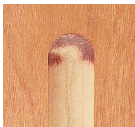
▲ Routing a stopped flute usually results in burn marks at the ends.
