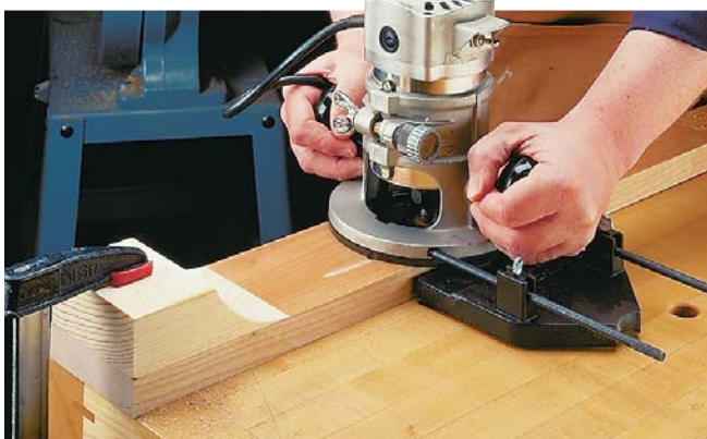
▲ Routing a stopped flute usually results in burn marks at the ends.
