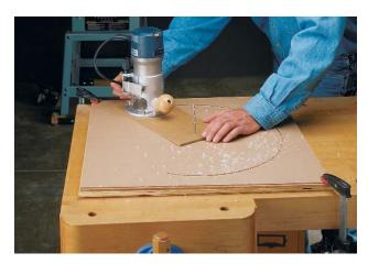
slightly wider than the base of my router.) Bore these holes and make sure to countersink the holes for the head of the mounting screws.
