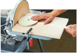
**Jig** – Basically, the jig consists of three parts: an MDF base, an adjustable hardwood runner, and a pivot pin
