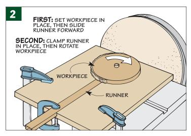
Note: The pivot pin can be any size you need. I have a set of runners with different size pivot pins. But depending on the dowels you use, you may find the fit a little loose. A quick way to solve this problem is to wrap the pivot pin with masking tape until you get a snug fit.
