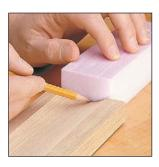
**1.** Trace profile First butt the foam block against the molding and trace the profile.
