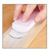
**3. Sand profile**Smooth the profile by rubbing it across a piece of sandpaper stuck to the workpiece.
