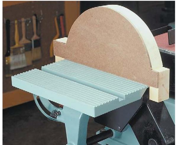
Next, I made a cover to hide the disc. I placed the completed arch assembly on a piece of hardboard and traced the profile down to the platform cleats. Then I cut out the cover on a band saw and glued it to the framework. Finally, I sanded the edges of the cover flush with the frame.
