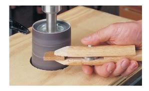
Here's how it works. A small hardwood wedge fits into the back end of the clamp. This allows the front jaws of the clamp to "bite" down on the object that is being held. The further the wedge is pushed in, the tighter the grip. A bolt and wing nut hold everything together.`
