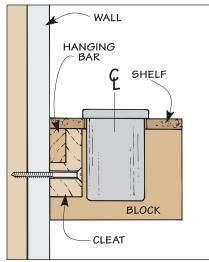
A block is attached to each end of the shelf. The two blocks prevent the caddy from tipping over when I set it on my workbench. Once the blocks are attached to the shelf, a shelf cleat is cut to fit between the blocks. To hang the caddy, the shelf cleat simply slips into a rabbet cut in the wall cleat.
