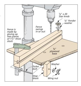
The base is just a piece of 3/4"-thick plywood that is mounted to the drill press table with carriage bolts, see detail 'b.'
