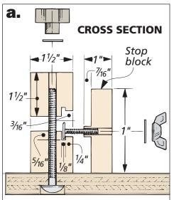
The stop block has a tongue that rides in the slot on the fence. To create the tongue, rabbets are cut along the top and bottom edges of the block. (To be safe, you'll want to start with an extra long blank.) Then a hole is drilled through the block to allow for a toilet bolt, washer, and wing nut.
