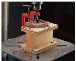
Completing the table is just a matter of drilling holes in the top and bottom pieces. This way, you can secure the table to the drill press with carriage bolts and a couple wing nuts. Make sure you bolt it in at least two slots to prevent the table from twisting.
