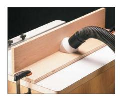
To attach the port to the fence I used some small  $\#4 \times 1^{1}\%$  Fh woodscrews. I simply drilled through the fence and into the reducer.
