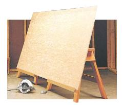
Another quick modification you can make is to add a simple L-shaped bracket to the side of each sawhorse. As you can see in the photo here, these brackets help to hold sheets of plywood so I can cut them down to a more manageable size. Because the plywood is held vertically, I don't have to stretch to cut all the way across the sheet.
