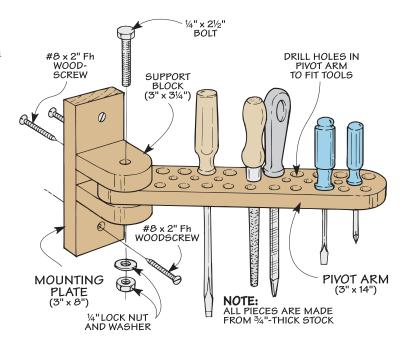
Before assembling the tool bar, I cut an arc on the outside end of each support block and on both ends of the pivot arm. This removes the sharp corners, and it allows the pivot arm to swing freely without binding. To create a pivot point, I used a bolt that passes through a hole in each support block and the pivot arm.
