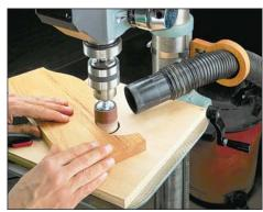
To allow you to tilt the yoke to the desired angle without loosening the wing nut, the hole in the metal clamp is slightly larger than the square shoulder of the bolt. And to provide clearance for the wing nut, there's a rectangular opening in the yoke. Finally, the large hole in the yoke is sized to accept the hose from the shop vacuum.
