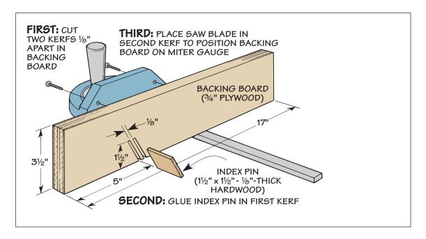
To use the jig, start by setting your blade to a 30° angle and cut one end of your featherboard. Then position the jig on the table, lining up the open kerf with your saw blade. Next secure the jig to your miter gauge with clamps or screws.
