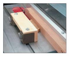
like the kind used to hold a dial indicator (above, left photo). We bought our magnetic bases from Enco Manufacturing. Search their web site <a href="www.use-enco.com">www.use-enco.com</a> for Part No. 625-0930 or call toll-free 1-800-873-3626 to order. **Note: magnets do not work on aluminum tables.**
