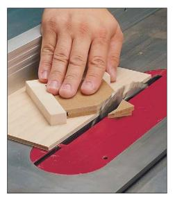
Using a table saw to trim a number of small parts to identical size can be tricky — especially if the cut is angled. But this small parts sled makes it easy and safe.
