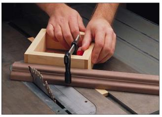
**The Jig** – To make the jig, cut four pieces of stock for the sides. Rabbet joints at the ends of two of the pieces help align them during glue-up, as shown in the main drawing. (Note: Size the pieces for the box so it clears the blade once it's attached to the runner, as illustrated in the detail at right).
