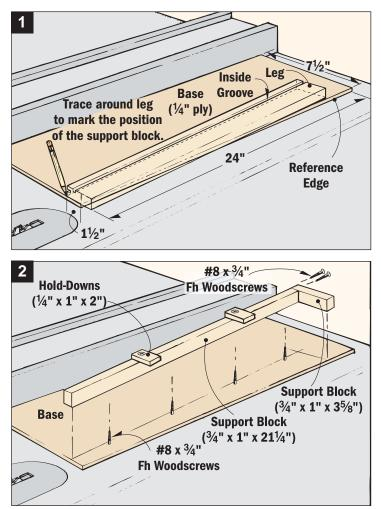
To build the jig, start by ripping a piece of plywood for the base. The ripped edge will serve as a reference to indicate the path of the saw blade. This same reference edge can be used to align the leg on the base and help locate the support blocks.
