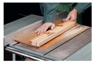
The jig is nothing more than a plywood base with two support blocks. The base acts like a "sled"
