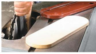
**SIMPLE PROCESS.** You can make one of these plywood inserts in short order. The drawings below show how to use the standard insert, first as a pattern, then as a routing template. This works great. Fig. a shows how to complete the job.
