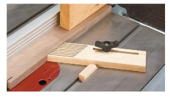
knob forces the head of the bolt into the slot and locks it down.
