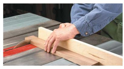
of the fence. This allows you to make your cuts with complete control of the workpiece.
