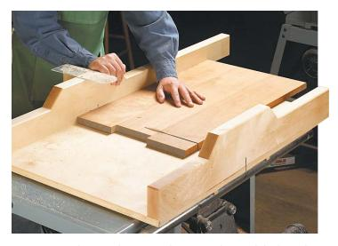
**USER NOTE.** When I make a cut, I always stand toward the left side of the sled and push with my right hand on the left top of the fence as you see in the photo above. My left hand is free to hold the workpiece flat and tightly against the fence. This makes control of the workpiece easier and the feed will be smoother.
