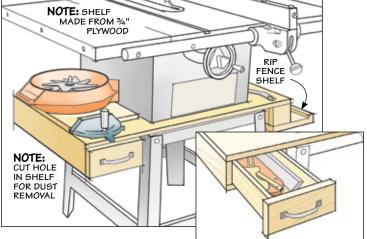
The second addition is a small drawer under the left side. Here I can keep push sticks, throat plates, and a few pencils and rules handy and dust free.
