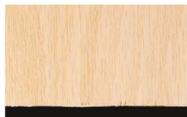
Attaching a "zero clearance" auxiliary base plate to the saw prevents chipout.
