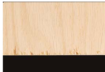
The blade on a circular saw tends to chip out fibers on the top side of the plywood.
