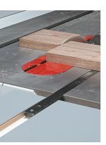
Miter Bar Slot. A dado slightly wider than the miter slot provides clearance for the miter gauge bar. An outfeed support should be stable enough and large enough to catch a workpiece as it slides off the saw. And this design fills the bill on both counts. The folding leg assembly and solid connection to the saw provide a strong base. And with the 18" by 36" top, you'll have plenty of worksurface.
